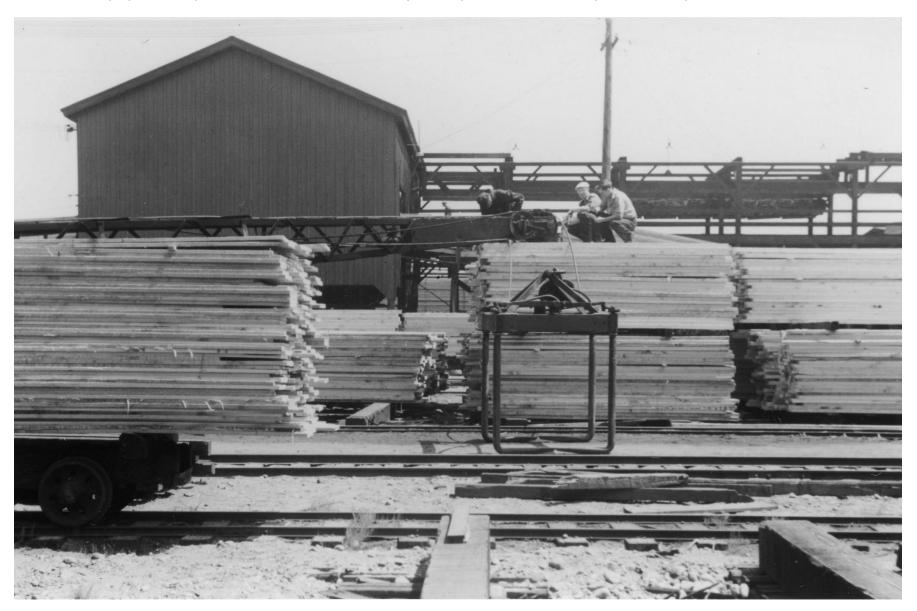
Steam-powered standard gauge traveling crane hoists a stack of lumber at Mill B, circa 1940. Note 30" gauge tracks crossing and parallel to standard gauge. Juleen Studio photo, courtesy Everett History Museum, 1995.4.62.
