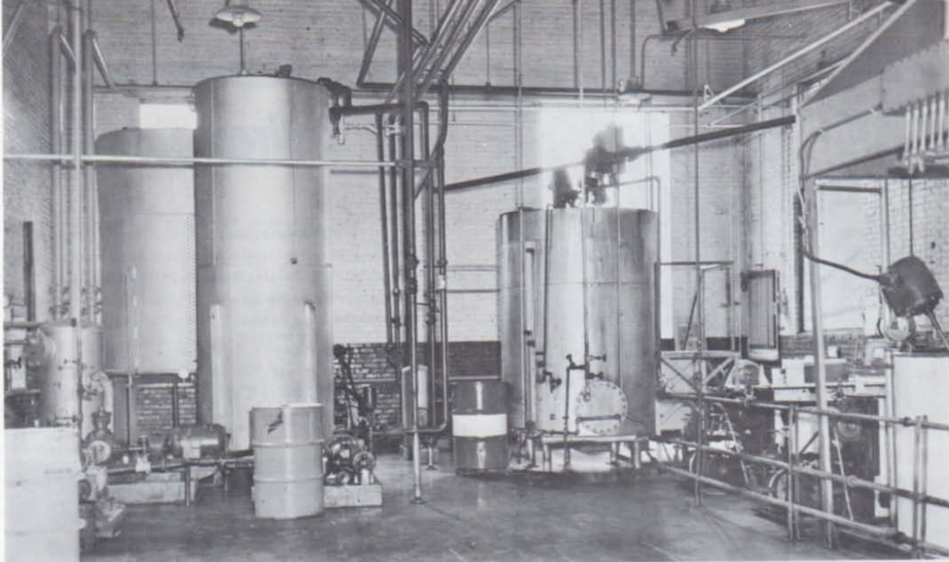
TOWERING TANKS, part of diesel oil processing system, stand out among maze of pipes and equipment at Livingston store's oil reclamation plant. Plant operates 16 hours daily, 5 days-a-week, re-refining four different types of diesel lubricating oil.
