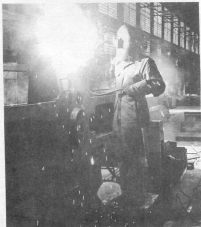
UNDERFRAME WORK --Welder joins bolster casting to underframe of boxcar. A shop-developed "turn-over" device rotates the nine-ton underframe a full 360 degrees to give unusually good welding angles.
