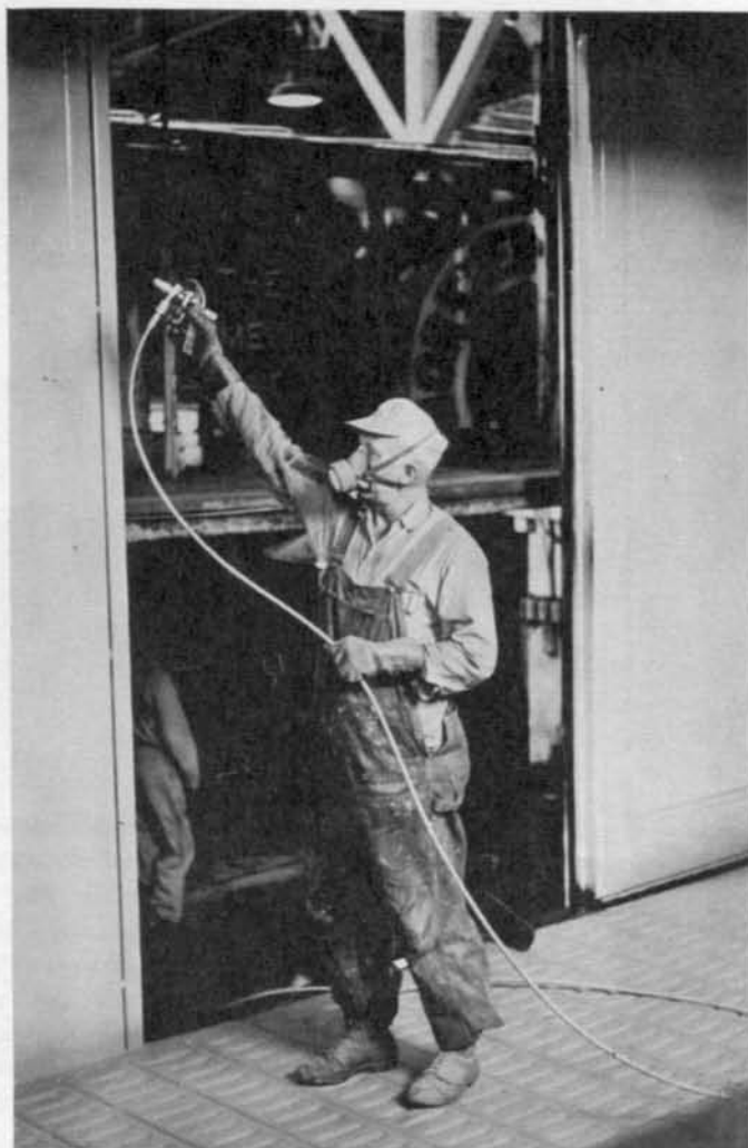
PAINT JOB --Completed box car is given once-over on its interior with special paint coating. All that's left now is the stenciling and weighing and another NP boxcar is rolled out of Brainerd shop.
