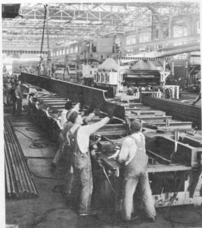
BOXCAR BEGINNING --one of 561 cars scheduled to be built at NP's Brainerd shop in 1963 starts to take shape. Here, side sill of car underframe is positioned in jig where air-operated clamps hold it for welding.
