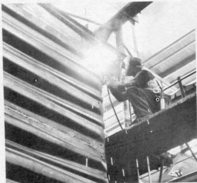
SIDES, ENDS JOINED --After boxcar underframe is mounted on trucks and has prefabricated sides butted onto it, a welder is lowered on a special platform to join sides and ends of boxcar with a continuous weld.
