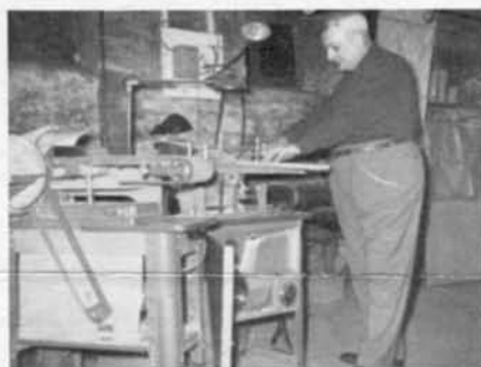
Here Cliff is shown operating the bench saw. Sander and sanding disc are in the foreground.
