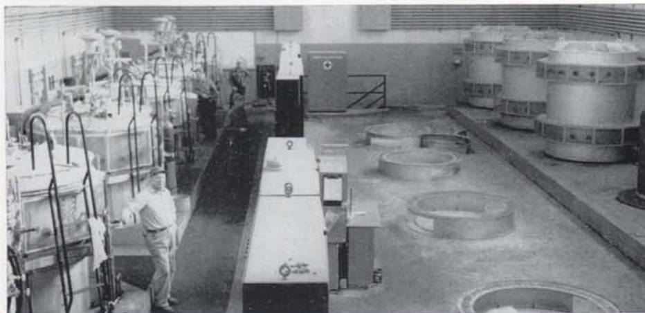
CARBON ELECTRIC FURNACES , left, at the Wah Chang corporation, are used in reduction of zirconium and hafnium, both of which occur in imported zircon. Distillation furnaces, right, also are required in refining processes at the plant.
