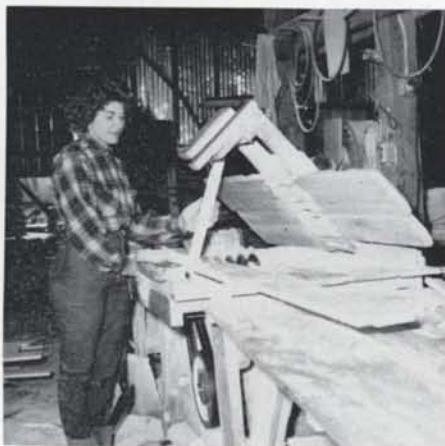
USING THIS HOMEMADE multiple rip saw, Jean Cash makes frames for louvers in Brookshier factory in Idaho.
