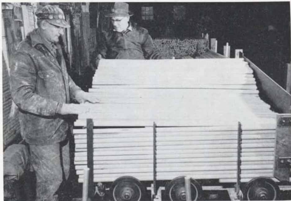
HANDLES FOR BROOMS AND MOPS seen here are ready to enter a sanding machine at factory of the St. Helens Wood Products company in Oregon. Nearly all are made from fir, but four other woods are used. Both sizes and colors are varied.
