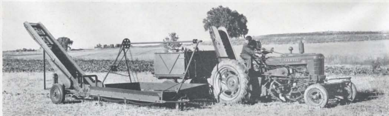
This view shows the topper and lifter, with holding cart in position to dump beets into stationary loader. The cart is tipped at one side, allowing beets to roll into hopper below it. This beet harvesting machinery is designed to serve growers with average size acreage and has enough capacity to harvest for two or three small growers in an ordinary season. It is considered still in the experimental stage.
