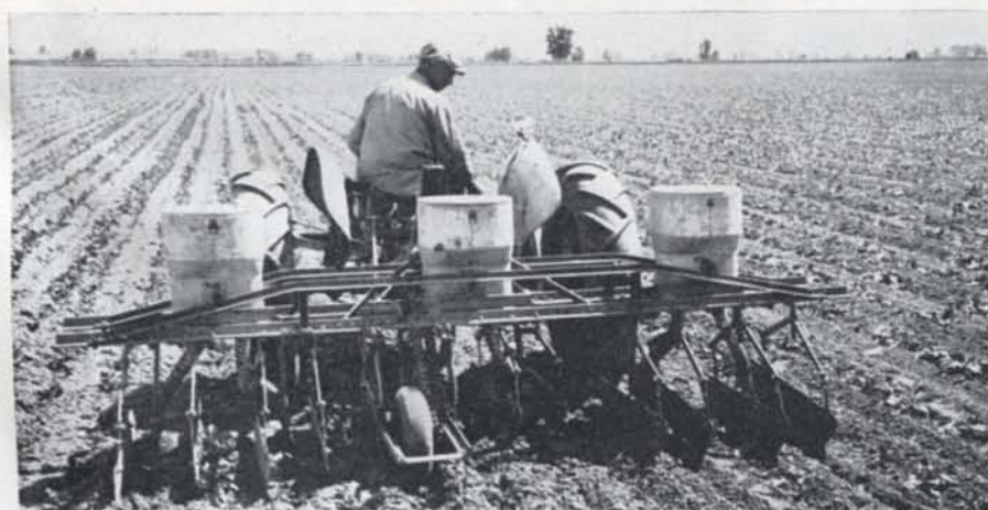
Western Montana sugar beet growers pepped up their fields with a couple of "shots" of ammonium nitrate fertilizer. As this material is quite soluble, it is put on, using attachment on the cultivator, as a side dressing while the crop is growing, when it will be used readily. Two hundred pounds an acre are applied in two applications of 100 pounds each. In the Bitter Root, Missoula, Lower Flathead and Toston-Townsend areas 2,675 acres were treated this year. The picture shows a six-row applicator, with cans mounted on cultivator. Later types, custom-made or built at home, have seven cans for six-row application.
