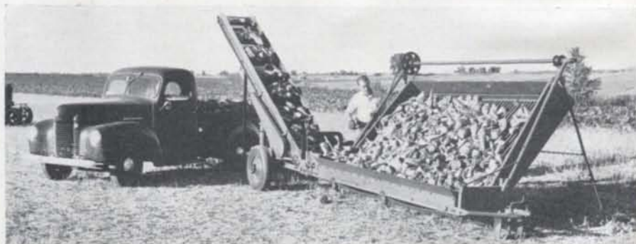
The stationary beet loader is a companion of the field machine. Tilted hopper, dumping into a conveyor and elevator, returns to horizontal position on the ground when it has disposed of its load. A three-horsepower engine powers this equipment, whose elevator moves faster than drag section.
