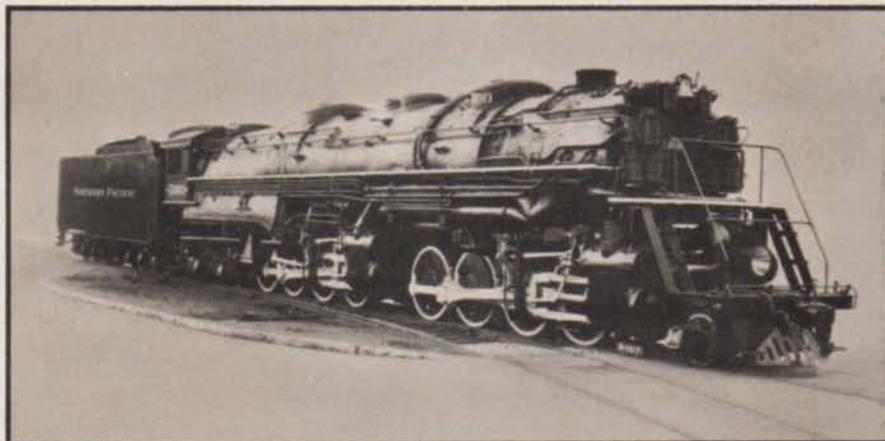
Known For Years as the "World's Largest Steam Locomotive," this 563-ton Yellowstone type was placed in service in 1929 in NP's mountain divisions. 125 feet long and over 17 feet high, it had twice the hauling capacity of locomotives used previously over this rugged terrain.
