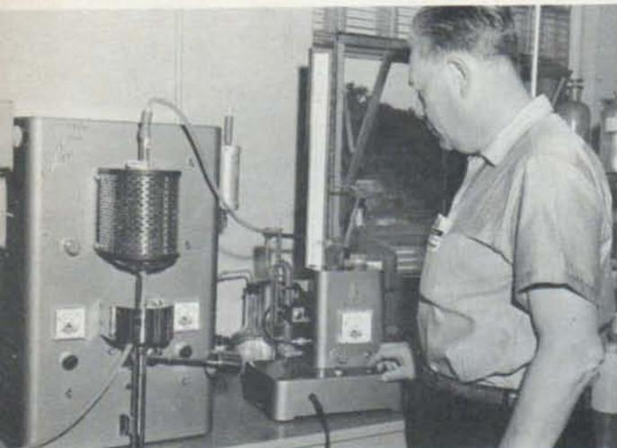
AT LEFT: Induction furnace enables rapid determination of sulphur content of fuel oil. Quality control is a major function of the Como (St. Paul) laboratory, which also has a branch for petroleum testing at Livingston, Mont. shop.
