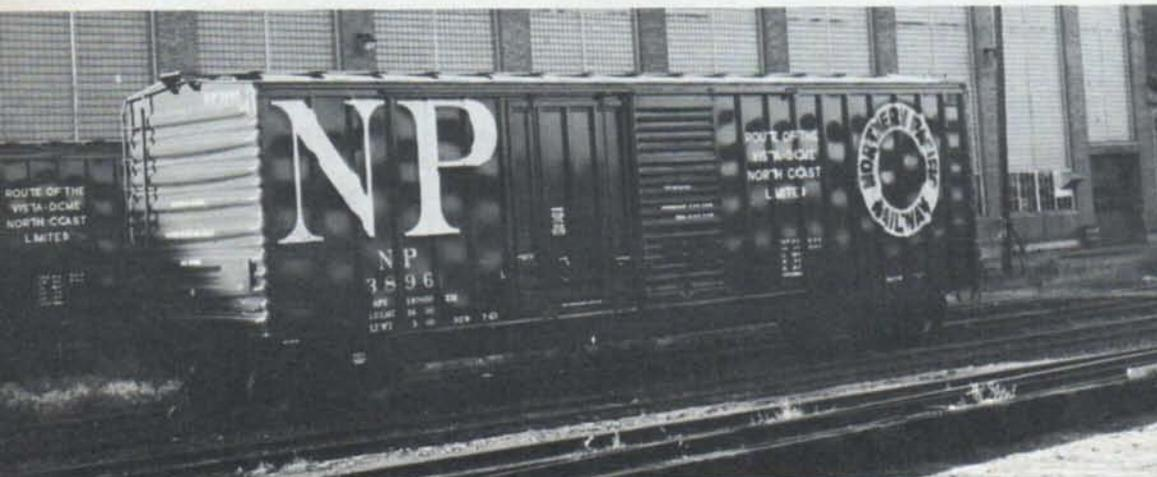
AT LEFT: Car shops are centralized on regional basis, with three heavy and nine "light" shops. Here at Brainerd, sides are placed on combination plug and sliding door boxcar. Car uses welded underframe with steel end castings.
