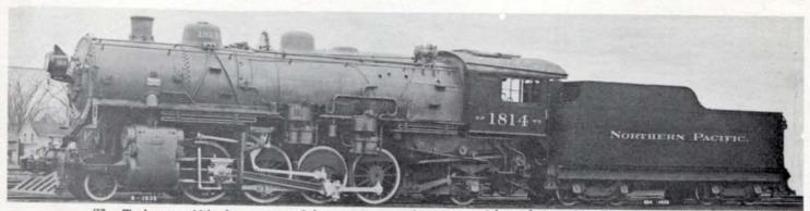
The W class or Mikado, was used for many years for main and branch line freight service prior to dieselization. The W-3 was built by American in 1920. It was 83 feet long, 15½ feet high and weighed 171 tons full loaded.
