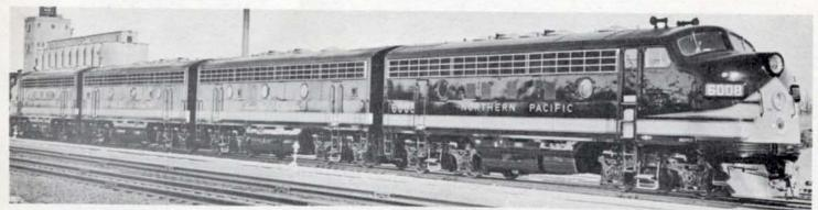
This locomotive has now replaced steam power for all main line heavy freight service. It generates a total of 6,000 H.P. from its 4 units, is 201 feet 4 inches long, 15 feet high and weighs 490 tons. It has 32 driving wheels. Later models generate 7,000 H.P.
