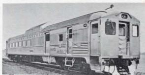
This is a modern, self-propelled car having air-conditioned accommodations for 48 passengers and compartments for mail, baggage and express. Built by Budd in 1955, three such units are now in branch line passenger service. Overall length is 85 feet; height 14<sup>1</sup>/<sub>2</sub> feet.
