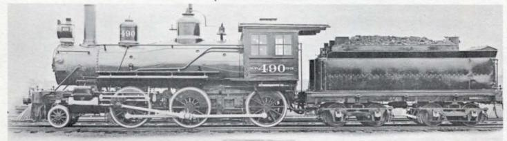
ROAD FREIGHT ENGINE CLASS D-3 2-6-0 The Mogul, running mate to the American Standard, this locomotive, built by Baldwin in 1889, was used extensively by NP for road freight service. It was 45½ feet long and weighed 52 tons.
