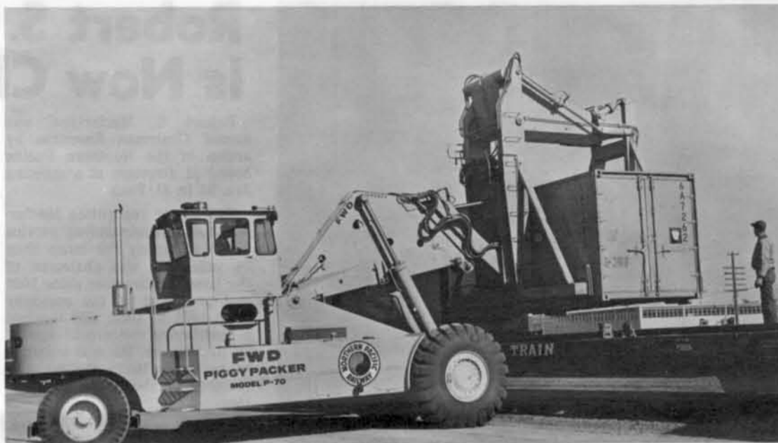
NP PIGGY-PACKER at Northtown Yards in the Twin Cities, unloads container unit from multi-purpose TTAX car. Loading and unloading operations each require only about five minutes. This container, one of 23 in the largest multi-container shipment handled in 1968 by Northern Pacific, is destined for Playhouse Company, Inc., in Minneapolis, loaded with toys.
