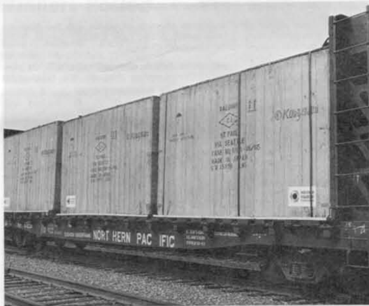
A GIANT ULTRA-FORMER used in the manufacture of varying thicknesses of paper was delivered to Hoerner-Waldorf Corporation at St. Paul in mid-July. The 600,000 pound unit, packed in special crates for sea movement from Japan to the Pacific Northwest, required seven bulkhead flatcars for rail movement from Seattle to St. Paul. The shipment is believed to be the heaviest unit ever handled as an import shipment by Northern Pacific. The shipment cleared customs in the Twin Cities.
