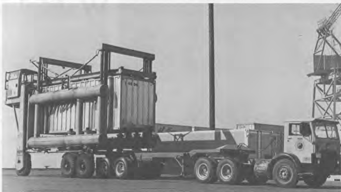
DOCKSIDE STRADDLE-TRUCK loads the first container aboard a new Northern Pacific container chassis at Seattle in new program.
