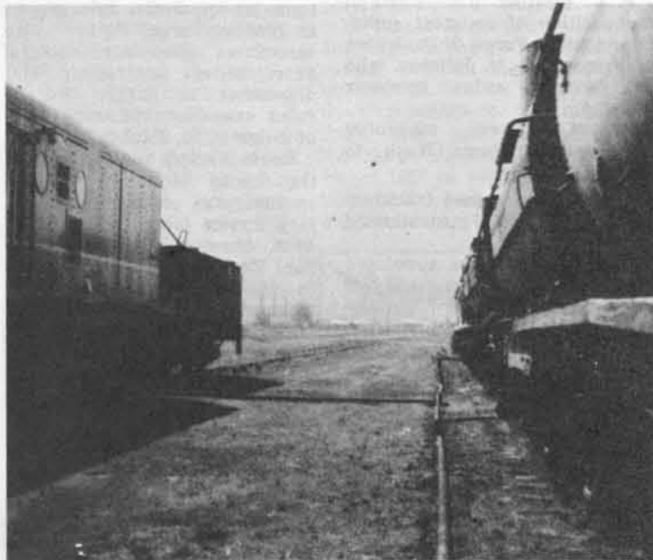
HEATER CAR at left provides steam at East Butte yard to keep asphalt in tank cars at nearly 300 degrees for pumping into Northern Pacific Transport Co. trucks which deliver it to tanks near highway construction zones.
