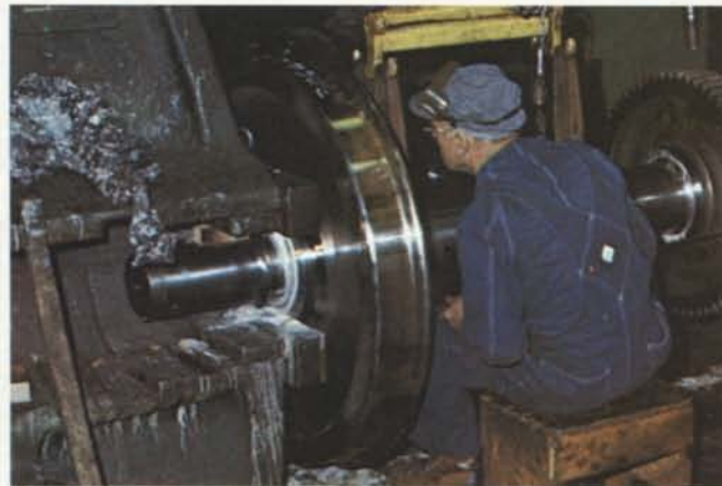
Del Miller controls air pressure on mount press as he and Phil Cummings assemble a pair of wheels.
