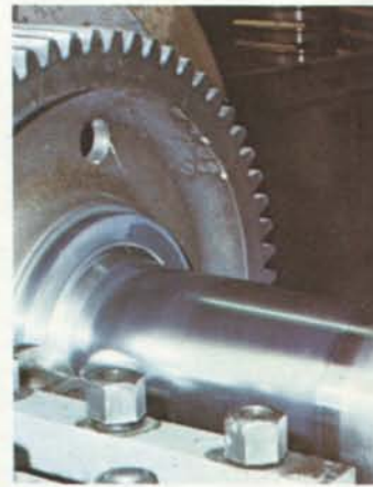
A close-up view of a wheel assembly in Wes' lathe shows shiny area he's rolling on the axle.
