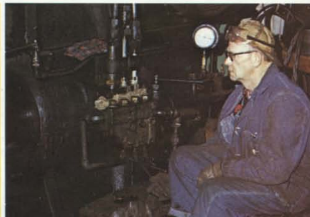
Del Miller controls air pressure on mount press as he and Phil Cummings assemble a pair of wheels.
