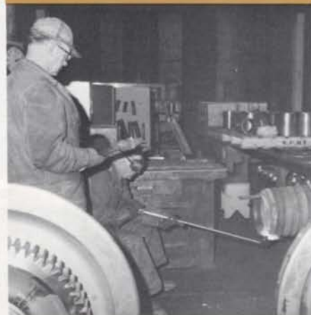
Phil heats up a water guard with a torch, then Del grabs it with his tongs to slip it on an axle.
