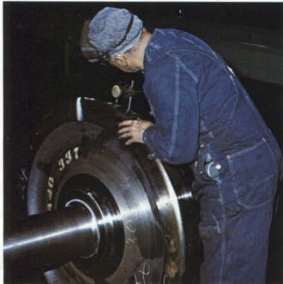
Wheels must be carefully measured with precision instruments to be certain they're perfectly circular.
