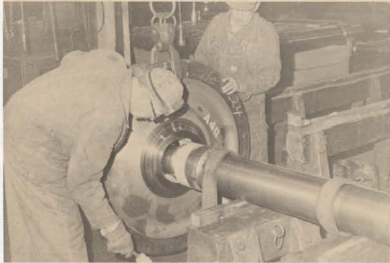
Phil heats up a water guard with a torch, then Del grabs it with his tongs to slip it on an axle.
