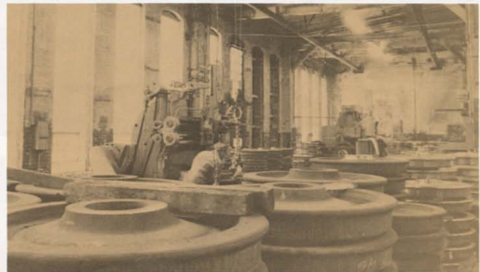
Vern Bohne is almost entirely hemmed in by stacks of new wheels as he bores hubs on some of them.
