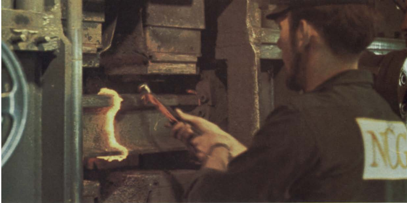
NCG man prepares to hook out excess steel after it's sheared off in box at right.
