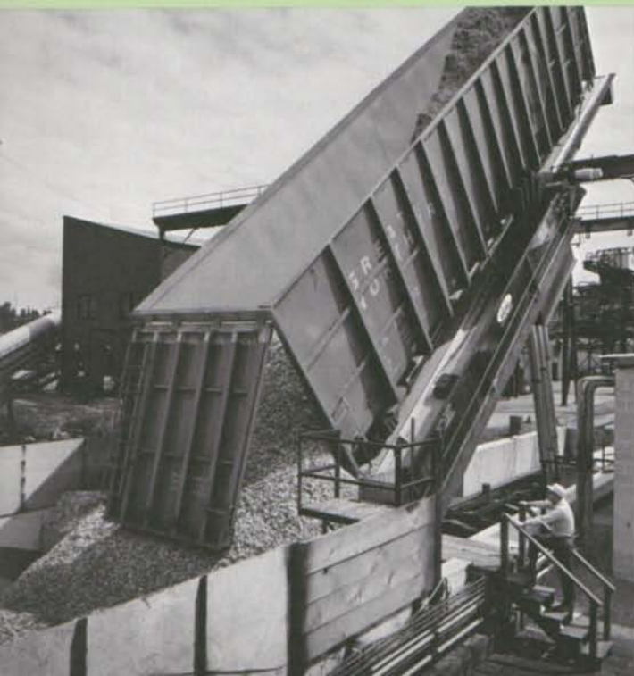
Hydraulic car tilting device speeds unloading at chip plant and maximizes use of wood chip cars.
