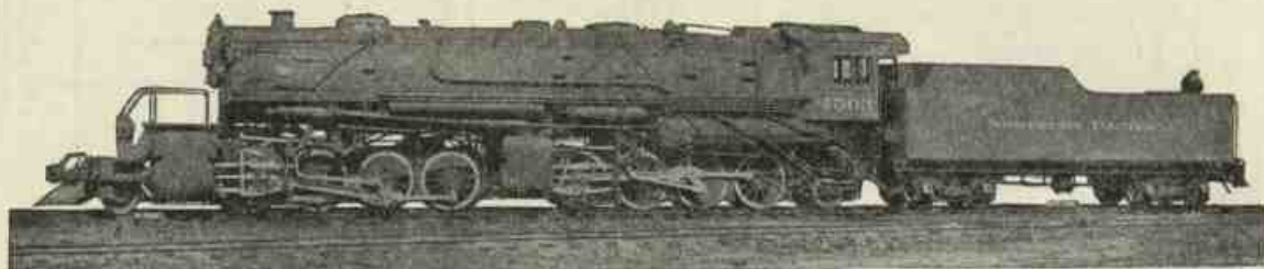
Giant N. P. Mallet Compound Locomotive—Tractive Power 107,300 Pounds
