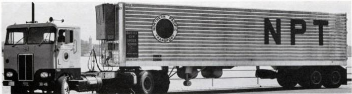
NOT ONLY RAIL EQUIPMENT but also motor power and trailers of the Northern Pacific and the Chicago, Burlington & Quincy will be brought together in the pending consolidation. The trailer pictured above is a new one owned by the Northern Pacific Transport company. The trailer has a propane-operated mechanical refrigeration system. It transports fresh and frozen foods.
