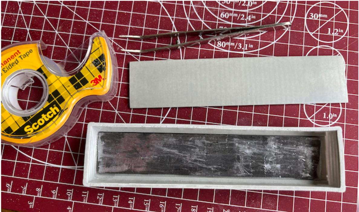
Fig. 10. Lead sheet weight taped into body casting, ready for floor casting to be affixed.
