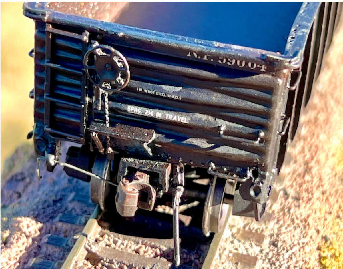
Figs. 15 a & b. Completed model, lettered to represent a car *ca.* 1969 as repainted in the early 1960s. Upgrades on the pictured model include A-Line metal stirrups and Archer Surface Details retainer clips applied to the upper side panels. This model was painted with Tamiya Fine Detail Surfacer primer, under an airbrushed coat of Tamiya acrylic blend of Nato black and flat black. The model was lettered with some decals from each of the two NPRHA sets for gondolas.
