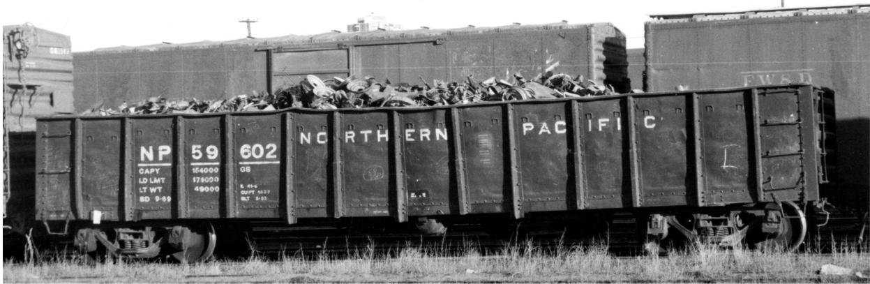
Fig. 7. NP 59602, a car rebuilt in 1967. Three elongate side posts, the square corner pieces and nonterminating ends are visible in this view.
