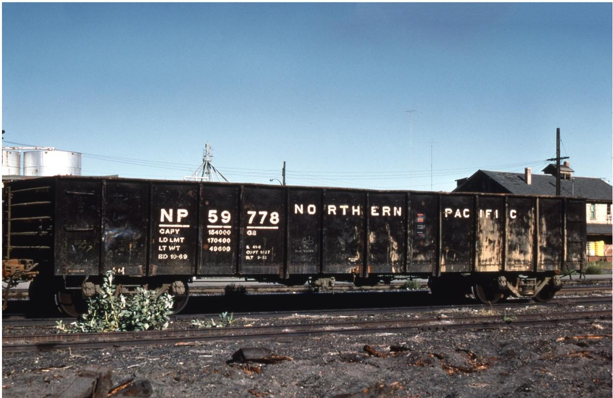
Fig. 8. NP 59778, another rebuilt car, with a view of the replacement end. This was “sort of” the standard lettering scheme for the rebuilt cars, though variants occurred. The Wallace cars with reinforced floors for example, lacked the horizontal underline below the reporting marks.
