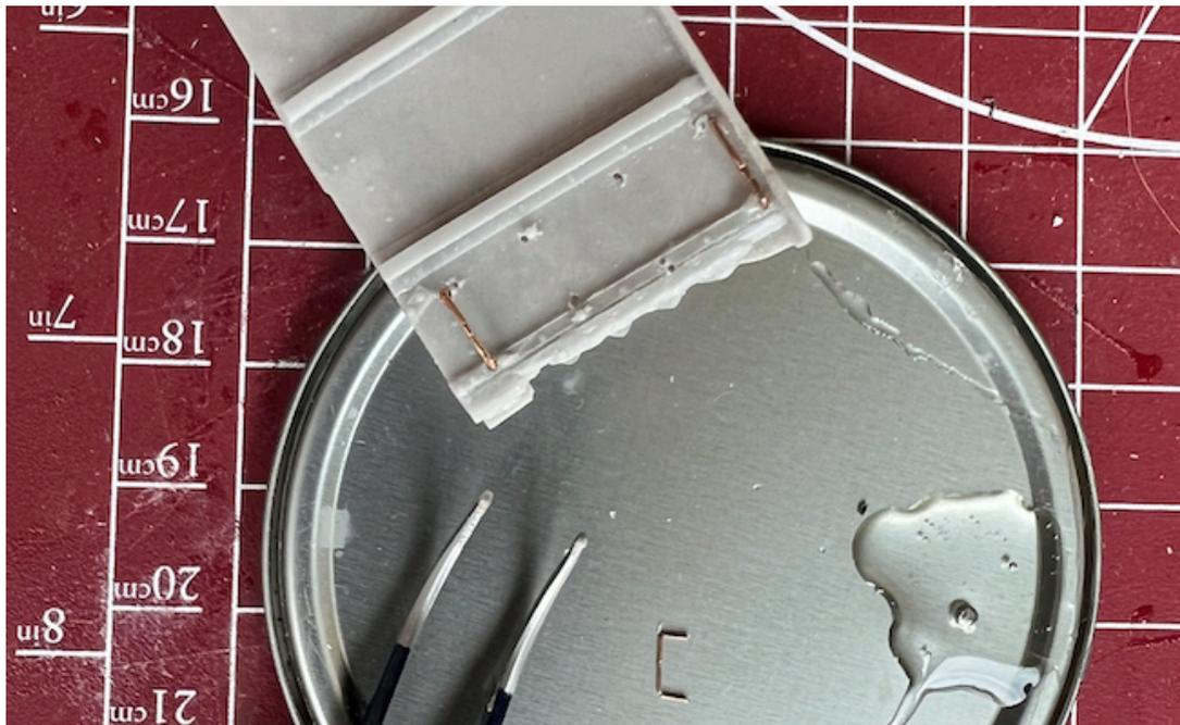
Fig. 11. Installing trimmed grab irons into drilled body casting.
