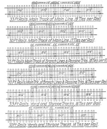
N.P.R.Y. Standard Plan of Tie Spacing for Broken Joints Plan T-16-102 Nov. 4th 1914
